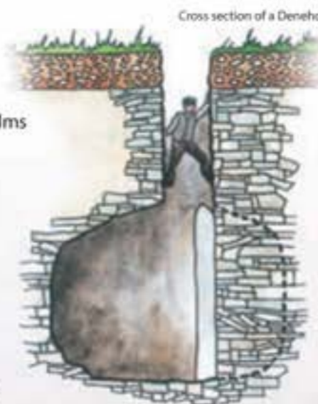
Cross section of a Denehole
