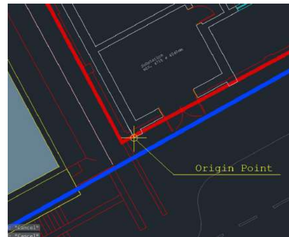
Origin point on corner of Block A
