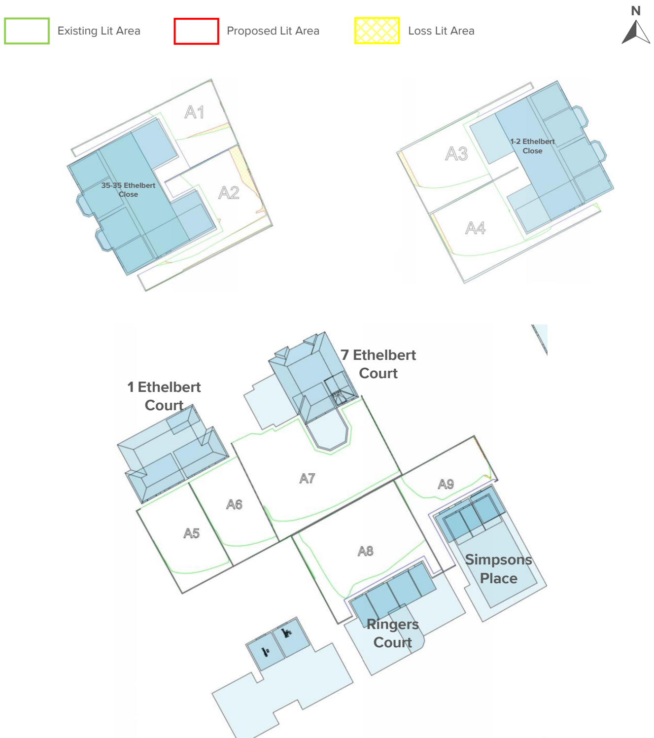
Figure 35: Overshadowing results for existing and proposed cases in amenity spaces.
