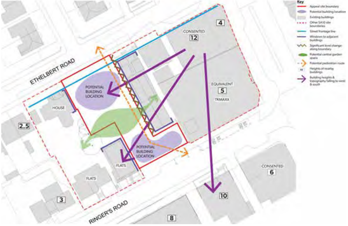
Fig. 3.15 Opportunities and Constraints diagram (by AR) for the appeal site locating it within the wider block's SA10 development area and noting the physical constraints - not noted anywhere in appellant's DAS. Larger scale plan in Appendix section 1.0.
