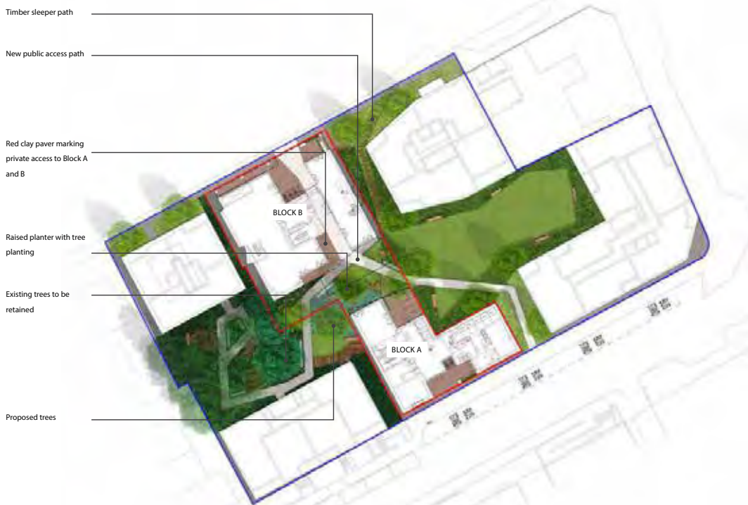
Fig. 4.18 DAS p.59 The landscape architect's design approach for the overall development of the balance of the urban block. As well as not reflecting the correct boundary locations around 66-70 High St (as with the architects), this does not take into account the level changes, in particular those between the appeal site and the adjacent Salvation Army site to the site's north-east.
