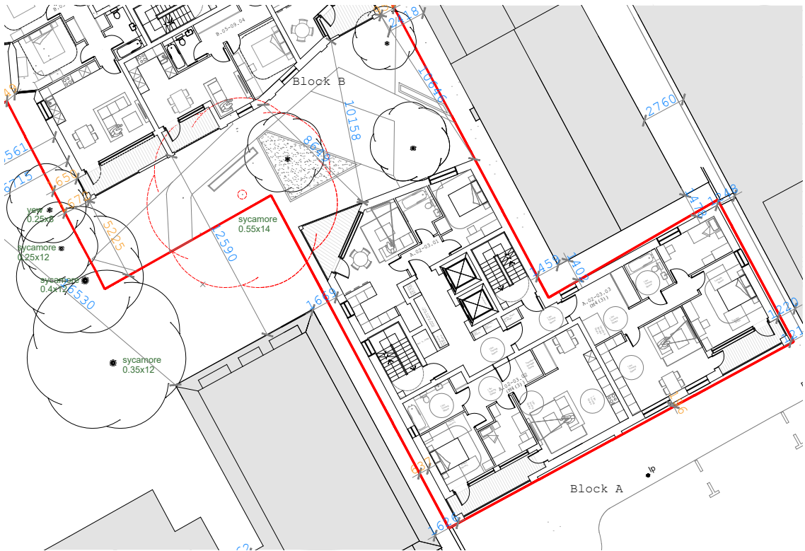
Fig. 4.4 Part plan (by Hollaway Architects Drwg no. 100.10) showing distances between appeal proposal building Block A and site boundaries as well as to immediately adjacent buildings and parts of Block B. The proposed building (Block A) includes windows on several boundaries to adjacent sites.
