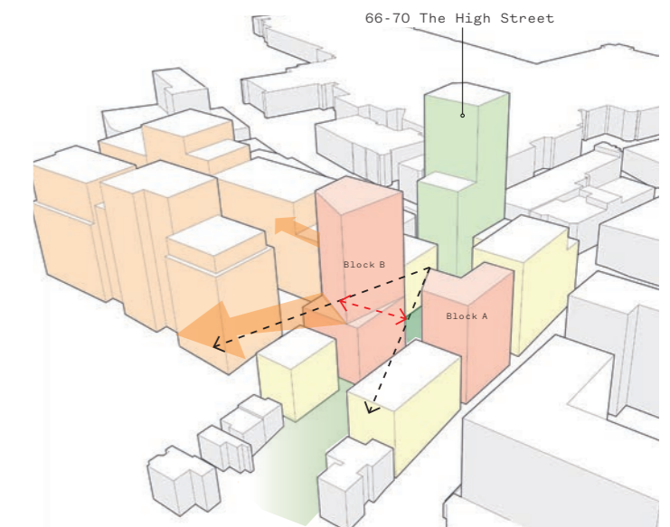
4. Angled Facade to Reduce Potential Direct Overlooking
