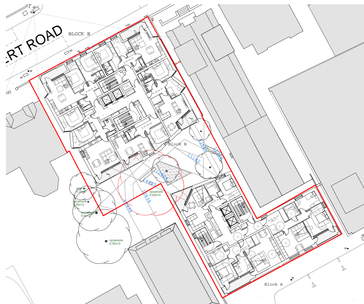
Diagram showing window to window separation distances on site, and floor plan layouts showing opposite room types.
