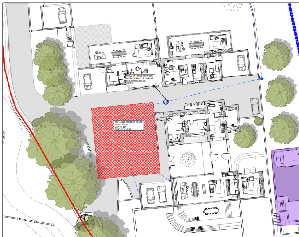
Figure 8.3 – Indicative drainage layout for the Polo Mews showing the geocellular storage tank.
