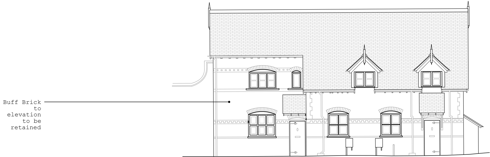
3&4 POLO MEWS - ELEVATION 1 EXISTING 1:100 @ A1
