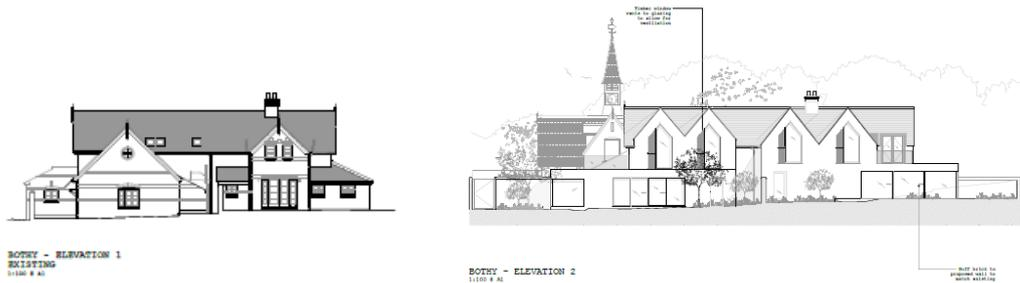
**Figure 12. Existing north elevation (left) and proposed north elevation plan (right)**
