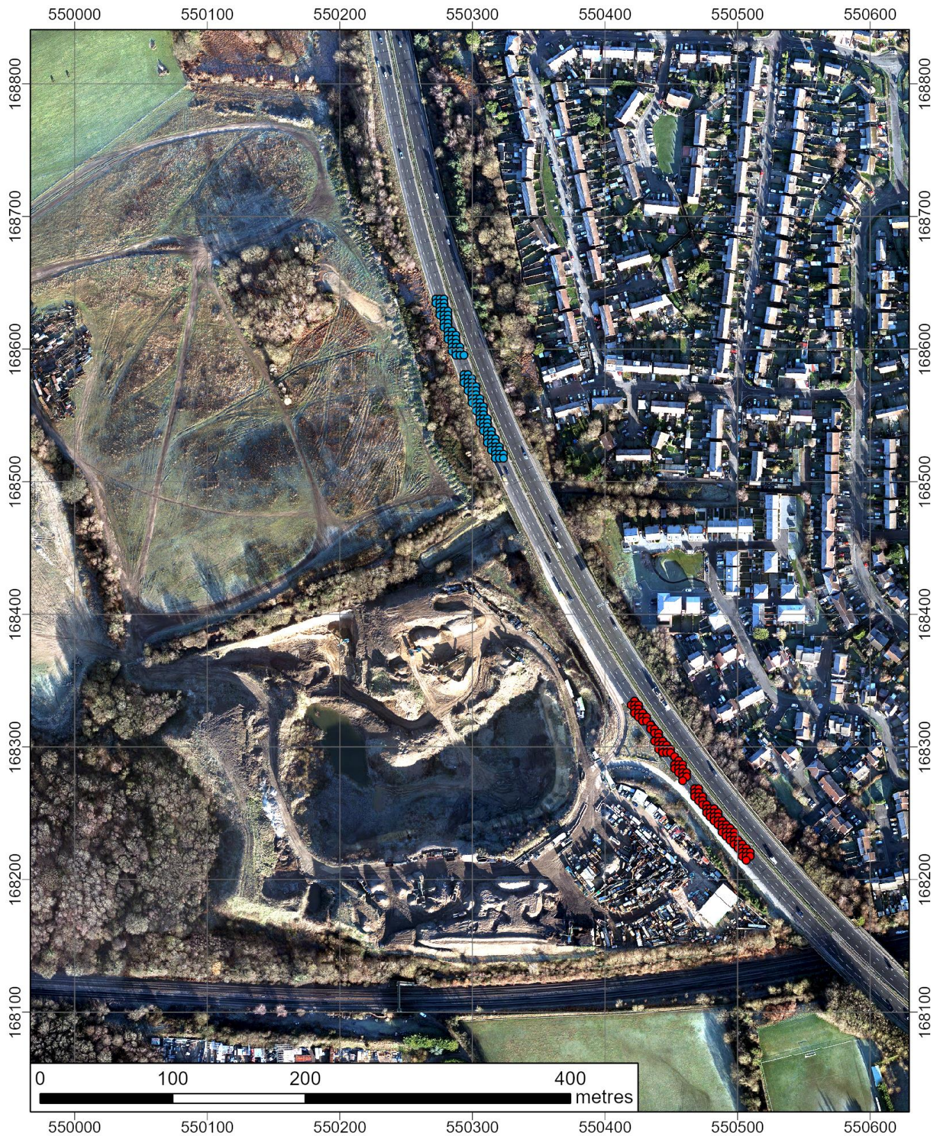
Figure 11 LIDAR sample points. Systematic error points in red, points used to estimate RMSE and confidence intervals in blue.
